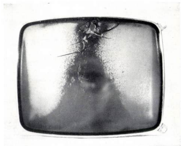
Fig. 11. Testing the new tube by the impact of a heavy steel ball on the tensile stress region of the bulb. The result is only a small hole and a few cracks in the face plate. Omission of the protective window is thus entirely warranted. The rapid ingress of air has blown away part of the fluorescent layer, as the photograph shows.
