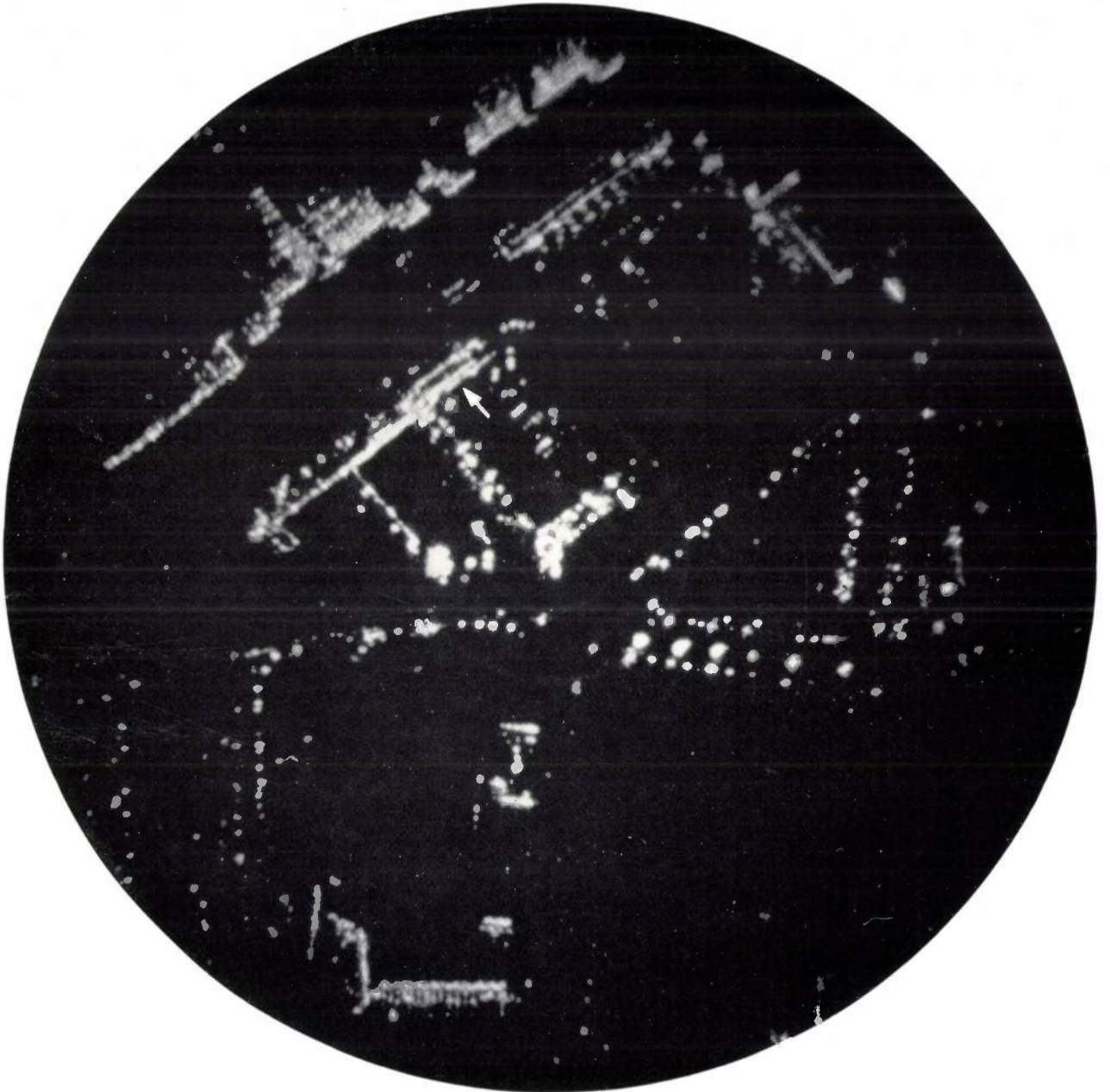
Fig. 13. The radar display covering the part of the town and the Philips factories immediately surrounding the Eindhoven Research Laboratories. The range was set here at 300 m.
