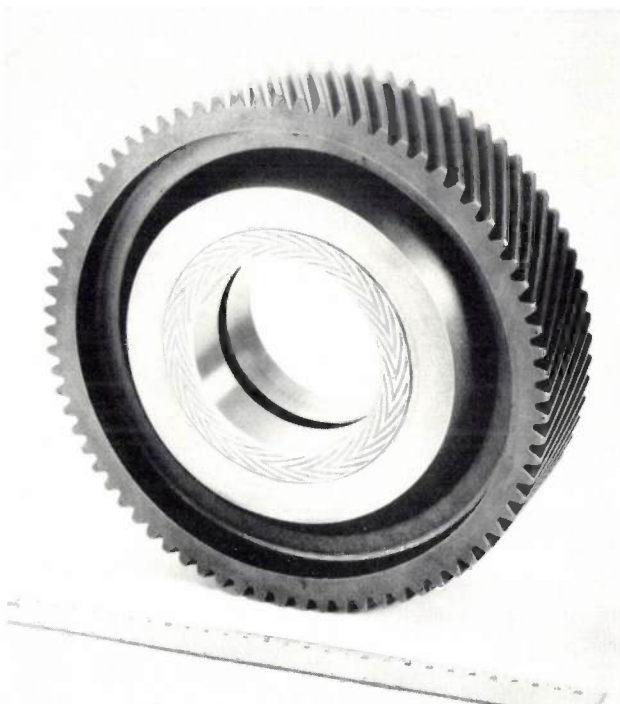
Fig. 25. A herringbone bearing employed in a hot gas engine developed in the Research Laboratories 21) .
