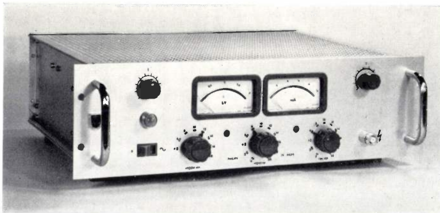
Fig. 1. The stabilized DC voltage source for 400-2000 V in a version that meets the same requirements as the apparatus described in this article, but which can supply a higher current, up to 10 mA.
