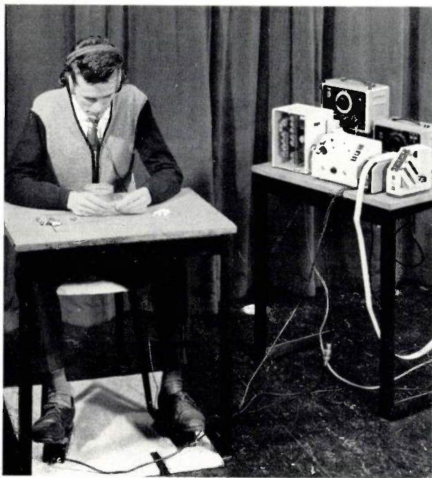
Fig. 11. The capacity meter developed in the Institute for Perception Research. In order to measure the difficulty of a perceptual task (here the assembly of a washer and a nut on a bolt), we investigate how the performance in this task deteriorates as the standard task is simultaneously carried out at a gradually increasing tempo. The standard task consists in depressing a pedal under the right foot when a high tone is heard in the headphones, and one under the left foot when a low tone is heard, the tones being produced in accordance with a random programme (on punched tape), at an adjustable rate. On the right, next to the punched-tape reader, may be seen the counter which records the number of correct reactions, and the number of errors sorted into two groups: reactions which come too late, and wrong reactions.
