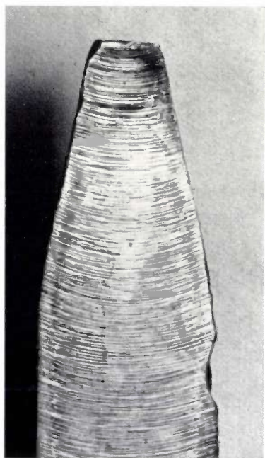
Fig.4. Longitudinal section of a crystal, with the striations made visible by pulsed copper-plating. (Growth direction from top to bottom; this is true of all the longitudinal sections reproduced in this article.)
